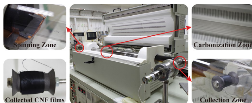
Figure 1. Continuous fabrication of carbon nanofiber films (CNF films) from carbon nanotube films (CNT films). Continuous CNT film is spun from a superaligned carbon nanotube array (SACNT array) fixed at one cold end of the quartz tube (labeled as spinning zone), through the hot zone heated by the furnace (labeled as carbonization zone), to the spool at the other cold end (labeled as collection zone). Pyrolytic carbon is deposited on the CNT due to the pyrolysis of the hydrocarbon gas in the carbonization zone. The collection of CNF films on the spool is driven by a dc motor. (Note that the photograph of the collection zone is mirrored; the width of the CNF films collected on the spool is 3 cm.)
